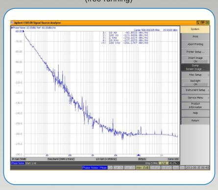
Figure 1: Typical Phase Noise Performance Plot for the 500 MHz MXO-PLD, P/N: 501-23950
